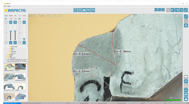
Weld bead inspection and measurements with INSPECTIS®
