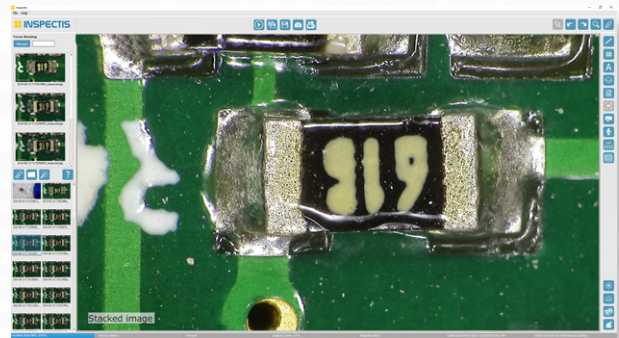
Resistor, focus stacked in INSPECTIS® ProX
