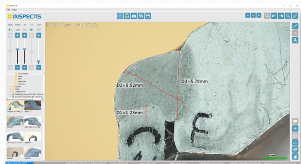
Weld bead inspection and measurements with INSPECTIS®
